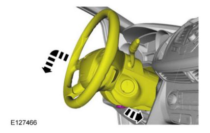
5. If equipped. Remove the retainer.
