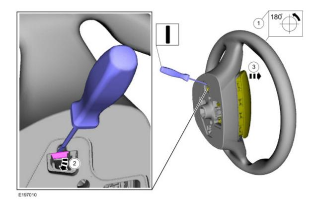
Disconnect the electrical connectors and remove the driver airbag.
