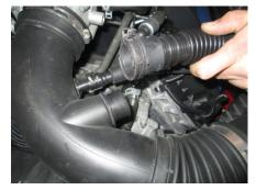
STEP 4: Remove bolt holding resonator tube to the frame rail. Remove tube from the bulkhead by pulling gently.
