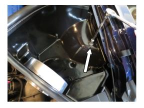
STEP 16: Install the provided weather strip around the perimeter of the newly installed air-box.
