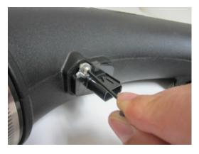
STEP 12: Install the provided grommet into the provision on the intake tube. Install the aluminum fitting into the grommet. A small amount of white lithium grease on the aluminum fitting will aid in the installation of the fitting.
