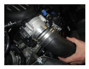
**STEP 9:** Remove the air-box retaining bolt. Remove air-box from car.
