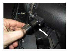
**STEP 3:** Remove intake resonator tube by depressing the hose clamp. Remove the tube.
