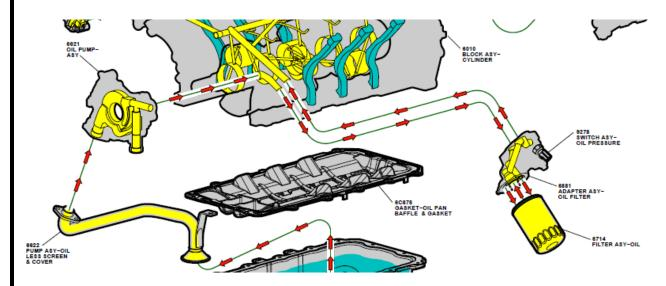
5.0L DOHC typical oil flow diagram
