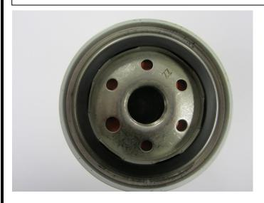
Center opening of the oil filter to block adapter port "A". Oil exits out of the oil filter from the center opening.
