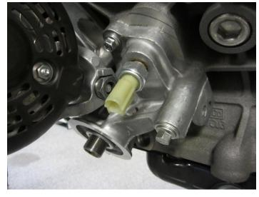
Check and note oil level on dipstick. With oil filter installed and full of oil, remove oil pressure sending unit. Using proper adapters, attach engine pre-lube tank to the port that the sending unit was screwed into. Following the engine pre-lube tank manufacturer's instructions, prime the engine.
