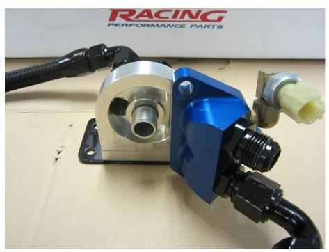
This picture shows the line attached to block adapter port "B" out to oil filter outside holes.
