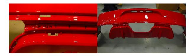
Step 26: Install lower valance by snapping into place and installing 3 screws on each side.
