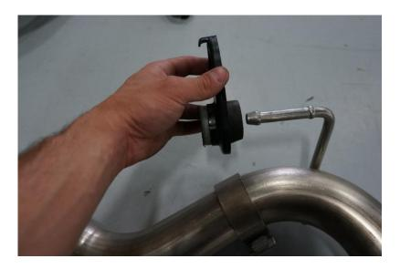
Step 10: Install supplied clamps onto x-pipe side of under axle pipes, slide pipes/clamps onto x-pipe. Using a 13mm socket install bolts in exhaust hangers in rear Sub frame.
