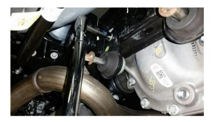
Step 12: Using a 15mm socket tighten nuts on x-pipe clamps 47.5 nm (35 lb-ft)
