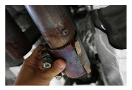
Step 8: Install new x-pipe onto clamps and tighten to 47.5nm (35 lb-ft)
