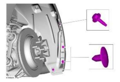
Step 17: Remove the bumper cover to bracket screws. (Two on each side) *Torque*: 13 lb.in (1.5 Nm)
