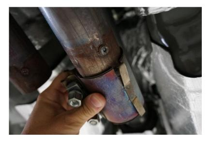
**Step 6:** Allowing exhaust to hang down, remove rear mufflers from hangers by moving the exhaust system towards front of vehicle.
