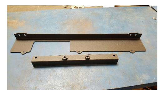
Note the long bolts with nut clips are for the front cross member mount. The short bolts will be needed to final install the rear skid plate to the add-on transmission support section. One bolt is shorter and has a small jam nut. That bolt must be installed on the right side under the wires to minimize chance of damage to the wire loom.
