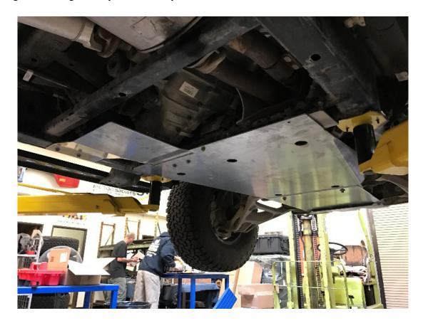
Move the large skid plate as needed until front and rear holes line up well. Re-install the factory bolts in the front section where the mid square skid plate matches up with the larger rear skid plate. Use the 2 outside holes even though this plate may have 3 holes. The center hole is left blank on this application.
