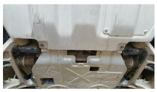
Remove the 2 bolts in the rear of the factory front skid plate. Remove the front bolts and remove the factory skid plate and keep all hardware for re-install later.
