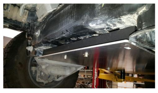
Locate the larger steel part that is installed over the transmission cross member. Remove the nuts off the transmission cross member bolts and slide the plate over the exposed bolts. Re-install the nuts with medium thread locking compound and torque to 76 lb. ft. to secure the cross member and the plate. When installing make sure the plate is aligned as it is in the photos.
