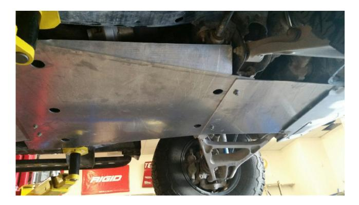
Locate the 3 small bolts provided with the kit. One is shorter and has a special short jam nut. Install the short bolt in the far right (passenger) side with the nut up. This bolt must be in the correct location so it will not rub on the wire loom that crosses over here. Put the other 2 bolts into the other 2 rear most holes.
