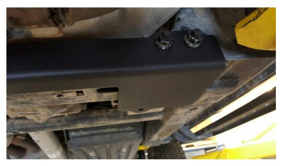
Locate the transfer case guard. The L shaped bent aluminum panel. Position this so it fits in the opening of the trans cross member section just installed. The bolts line up with the factory nut clips. Don't put bolts in the cross member now. **USE MEDIUM THREAD LOCKING COMPOUND ON ALL RE-USED FASTENERS**. Find the factory hardware and put the bolts in the frame mount side to hold the plate in place. Snug, but don't tighten yet.
