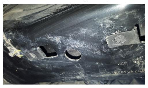
Locate the mid skid plate square section and the square tube cross member. Use the long bolts to attach the skid plate and square tube cross member. The aluminum plate has round holes and oval shaped holes. The oval holes go toward the front of the truck and these are the center holes you should use now. Put the long bolts in the 2 holes, but don't tighten yet. The square tube cross member has 2 spacers that are on the top when installed.
