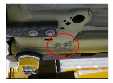
Identify the two provided tie down brackets with hole spacing that matches the holes left after bolts were removed. After applying blue threadlocker to the provided M10 bolts, install the forward two tie down brackets as shown below. The loops will point FORWARD. Torque bolts to 55 ft.lbs.
