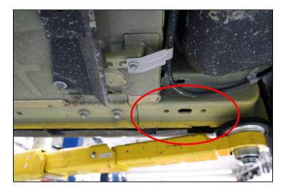
Step 5: After applying blue threadlocker to the provided bolts, install the remaining M10 bolts and rear two tie down brackets as shown below. The loops will point REARWARD. Torque bolts to 55 ft.lbs.
