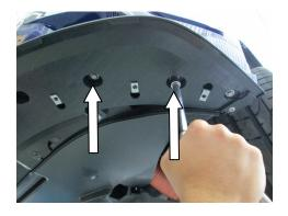
STEP 16: Place splitter against the bottom of the fascia, install (4) M8 x 45mm bolts into the locations noted in STEP 15 and torque bolts to 28 in.-lb.
