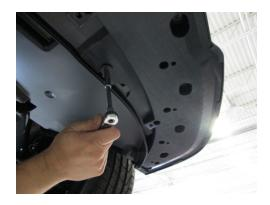
**STEP 3:** Remove the (2) outboard bolts securing the outside of the deflector.
