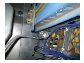
STEP 20: Install the deflector by sliding it forward verifying that its forward most lip is above the newly installed splitter.
