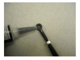
STEP 10: Apply a liberal amount of Blue thread locking compound on upper stanchion thread and proceed with installation. Install upper stanchion without support rod into the bumper bracket and tighten. This is done from below the vehicle, behind the lower grill.
