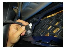
STEP 7: From the backside of the fascia, gently unclip the lower grille retaining clips from the fascia (12) locations. Remove the lower grille from the vehicle.
