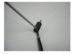
**STEP 9:** Apply RTV Silicone to the (2) Phillips screws covering threads and fill both eyelets.
