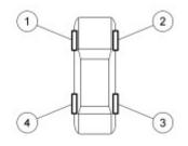
**STEP 8: NOTE:** *Do not wait more than 2 minutes between training each sensor or the <u>BCM</u> will time out and the <i>entire procedure must be repeated.*
