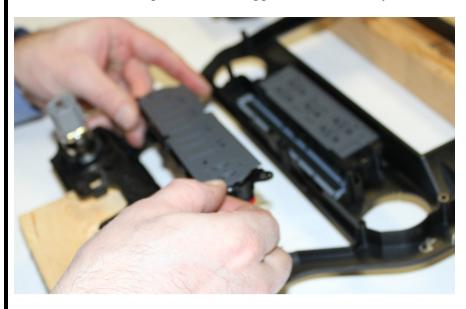
24. Remove the engine start and toggle switch contact pad
