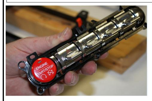
28. Reinstall the engine start and toggle switch assembly
