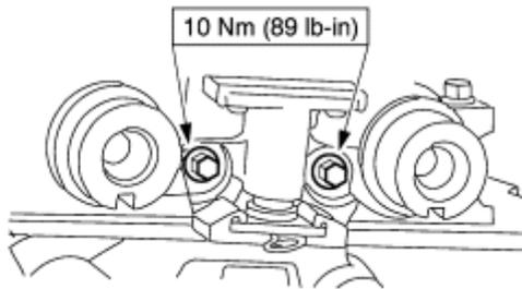
**STEP 2:** Install the camshaft sprockets and the chain as an assembly.
