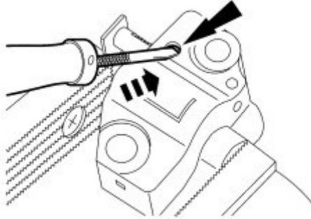
**STEP 5:** While holding the ratchet mechanism, push the ratchet arm back into the tensioner housing.
