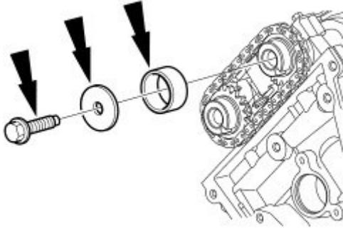
**STEP 5:** Install the camshaft sprocket, washer and bolt, and hand-tighten the bolt.
