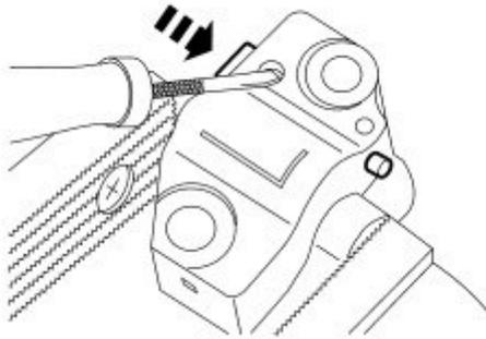
**STEP 6:** Insert a paper clip into the hole of each tensioner housing to hold the ratchet assembly and plunger in during installation.
