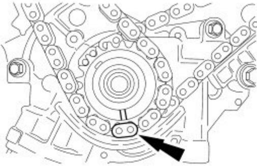
**STEP 19:** Install the RH timing chain onto the crankshaft sprocket, aligning the copper (marked) link with the timing marks on the sprocket.
