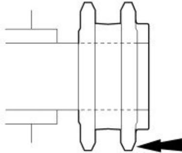
**STEP 13:** Position the LH (inner) timing chain on the crankshaft sprocket, aligning the copper (marked) link with the timing mark on the sprocket.
